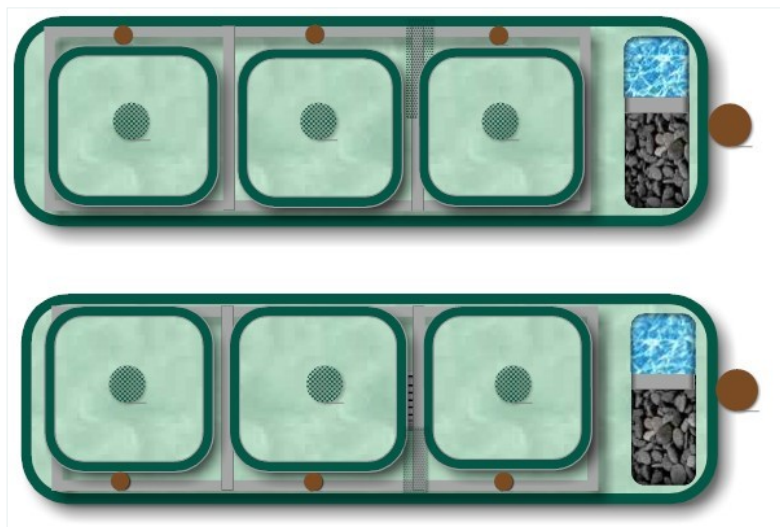
Fig.1. The hatcheries main elements are two identical units; each unit has a large fiberglass tank with three smaller tanks inside. Dimensions of the large tanks about 6.0 x 1.9 x 1.1 m (L x W x H). Dimensions of the smaller tanks are about 1.3 x 1.2 x 0.7 m. Each unit has the same equipment and can be operated independently from each other, which allows, for example, rearing trials with different water temperatures.
