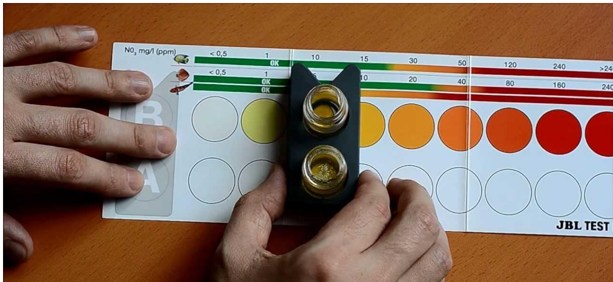
Fig. 28: After the given time, the tray with the two vials gas has to be placed on the related colour card (for each parameter, a specific colour card is available). The blank is put on the coloured spots, the sample on the white spots. Move the tray to the position where both vials show the same colour and read the value. Each colour card provides a recommendation for a safe range.
