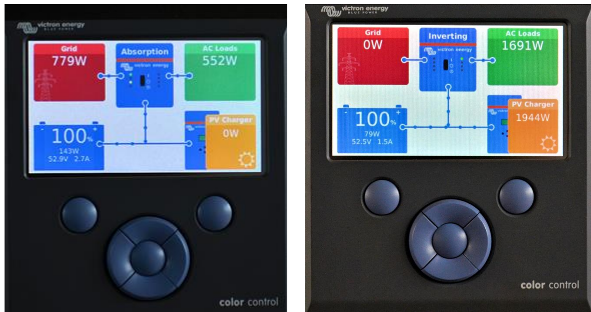
Fig. 5: Colour control of the Solar power facility. The monitor informs about the actual battery capacity and the flow of energy. Left: the hatchery uses mainly grid power, no solar energy available (e.g. in the night). Right: the hatchery uses power from the solar panels and the batteries. An important information for proper management of the battery capacity.
