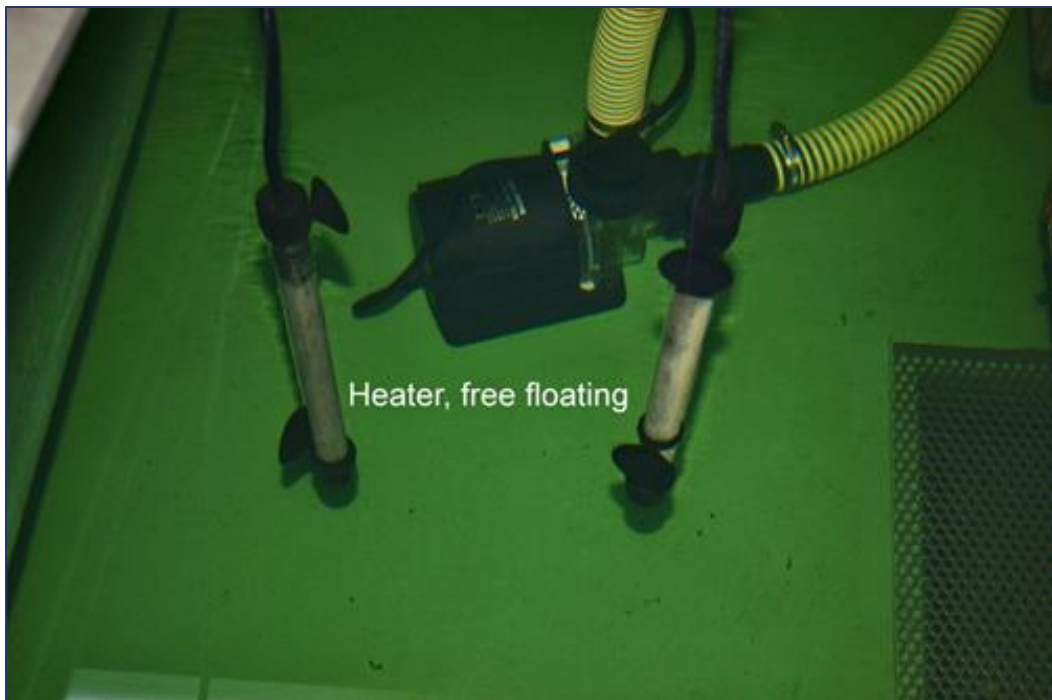
Fig. 16: Heater in the big tank. Please make sure that they are always well submerged and free floating without touching other devices.
