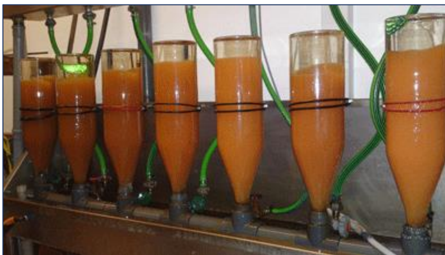
Fig. 30: Zuger glasses or Zuger jars are a type of equipment to breed fish eggs. Funnel shaped glasses contain the eggs while water is supplied from the bottom in an amount that the eggs are just kept in motion. The hatched fish larvae are usually collected with the spill over water from the top. Please note the high density of eggs which can be accommodated in the jars.
