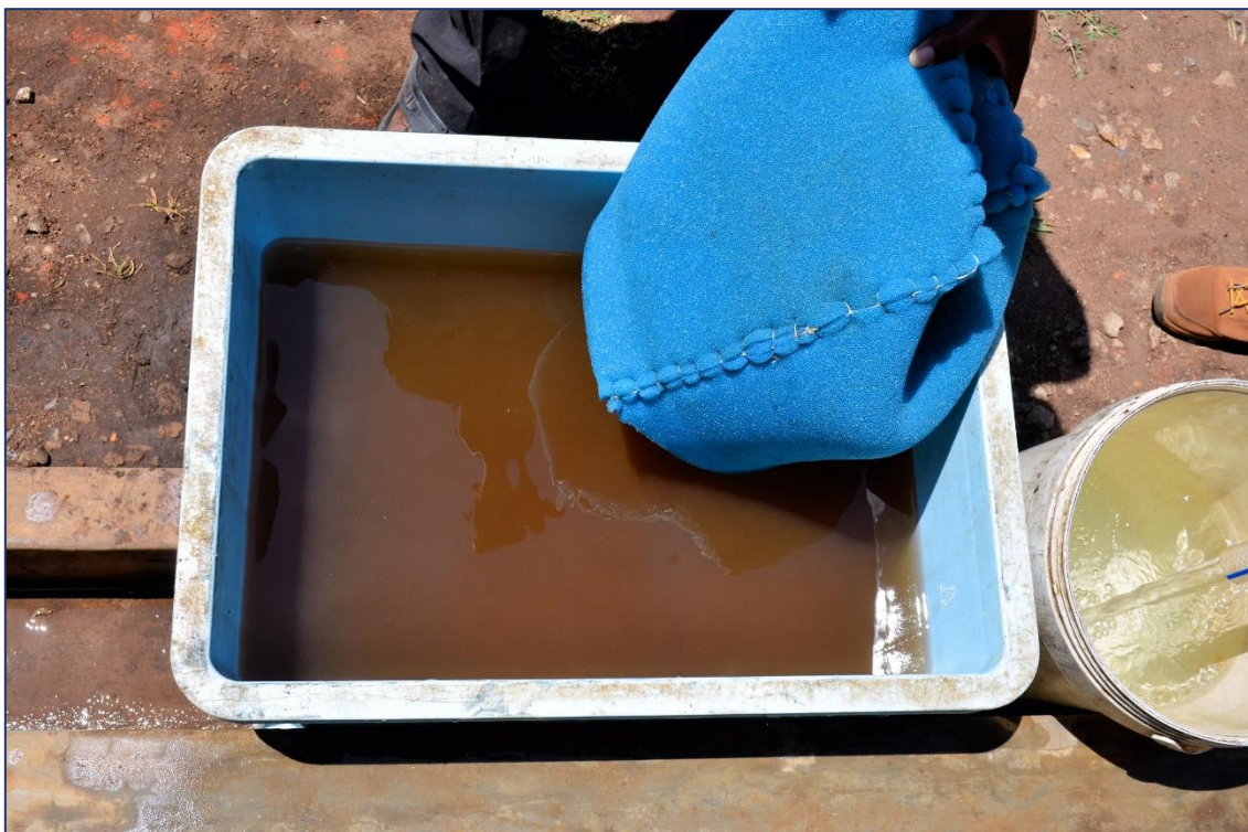
Fig. 24: The picture demonstrates the efficiency of the filter. This was the colour of the water after the first cleaning procedure. Continue until the water is almost clear. Put back the foam into the filter box, adjust the yellowish pipe into the foam box and re-start the pump.
