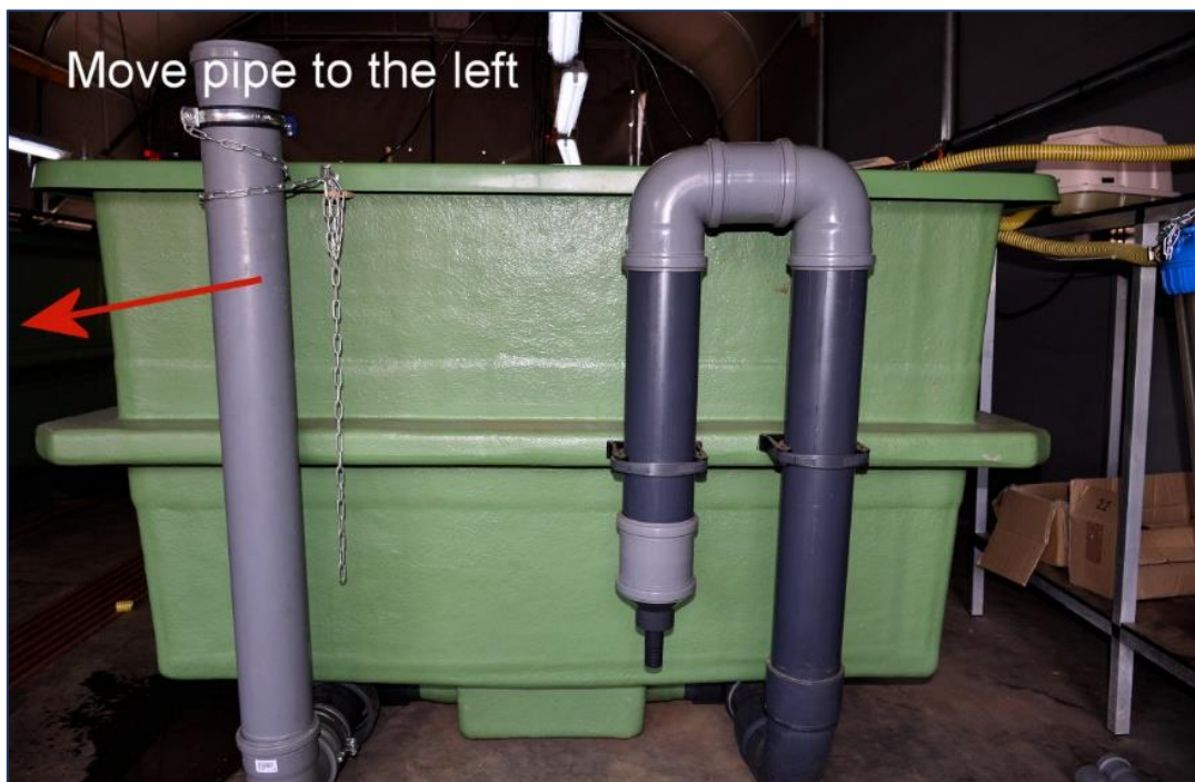
Fig. 19: The picture shows the outlet pipes of one of the units. The left pipe is used to drain water from the big tank. Remove the chain and turn the pipe slowly to the left until the desired water level after draining is adjusted. Secure the pipe with the chain and let the water drain out of the tank until the desired level is achieved. After finishing the draining process, put the pipe back to the default position as shown in the picture. Do not forget to fix the position of the pipe again with the chain. The pipe on the right side can be used when a flow-through set up is desired. The water which runs continuously out of the tanks can be collected with a tube to e.g. water plants.
