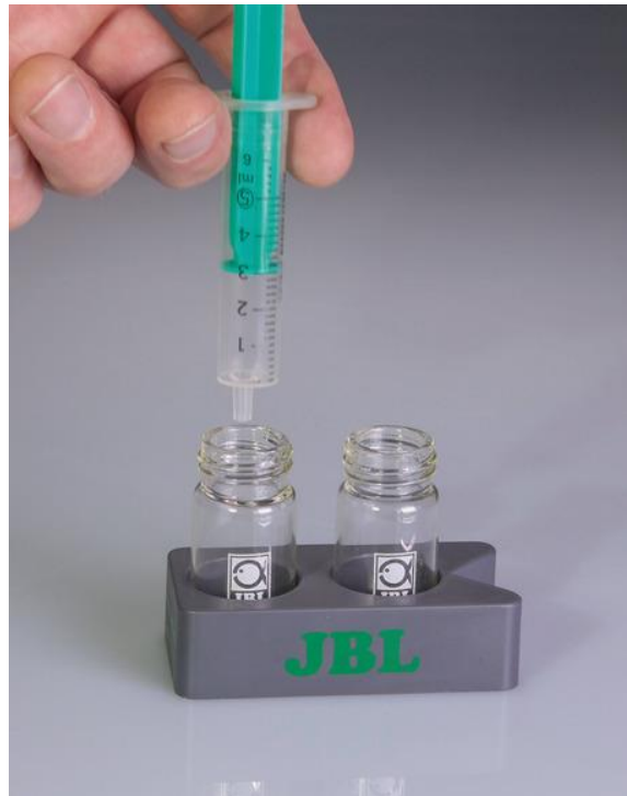
Fig. 26: Usually, two small glass vials are needed for a measurement. Both vials are filled with the water sample. In one vial reagents are added according to the manufacturers advices and some time is needed to develop the reaction (the colour).
