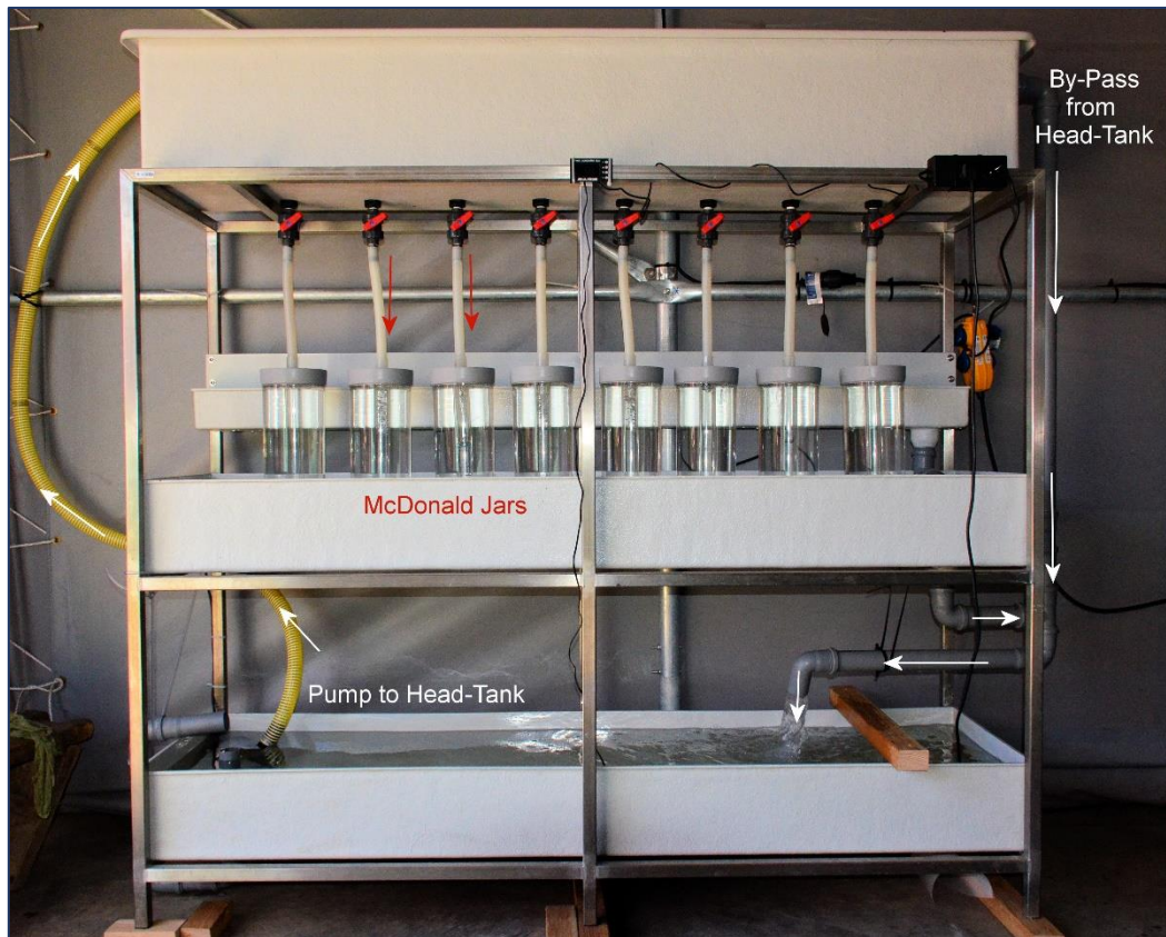
Fig. 29: Mc Donald unit, installed in the hatchery. The system has a head and bottom tank, a tray for the jars and water is pumped continuously from the bottom tank to the head tank. A 300-Watt heater is installed in the bottom tank to achieve an appropriate temperature (optimal temperature is supposed to be 28°C for e.g. O. karongae ). Flow through the jars can individually be adjusted.
