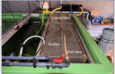
**Biofilter/Filterboxes.** The water to the biofilter is bypass water from the circulation through the rearing tanks. The amount of water which passes through the biofilter can be controlled with a ball valve and needs to be adjusted according to the efficiency of the biofilter (refer to ammonium measurements).
