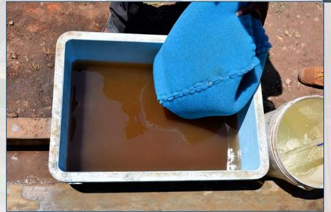
The picture demonstrates the efficiency of the filter. This was the colour of the water after the first cleaning procedure. Continue until the water is almost clear.
